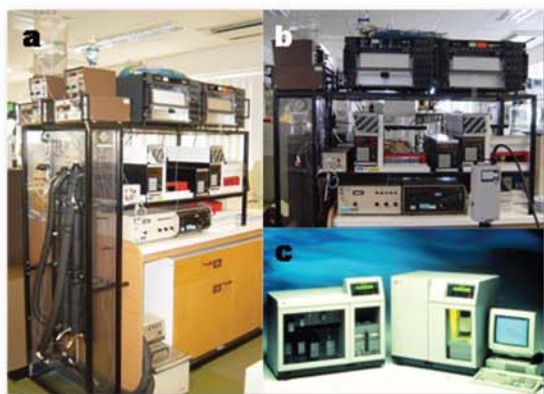
Figure 2. Development of automated carbohydrate release separation and sequencing. (a) The gel-permeation chromatography ('P4') system at the Oxford Glycobiology Institute, note heated water jackets, dual tritium and refractive index detectors, chart recorders and 1 m columns (1992). (b) Fraction collection for manual enzymatic sequencing. The output from the column shown in (a) is collected, and peaks are pooled and subjected to separate exoglycosidase digestion. This could take several months to complete (1992). (c) Left: GlycoPrep 1000, the first automated carbohydrate analysis system in the world developed by Oxford GlycoSystems from the technology of the Oxford Glycobiology Institute (1992). Right: RAAM (Reagent Array Analysis System) 2000 automated carbohydrate sequencer incorporating miniaturized column system with automated flow control, fluorescence-detection system and computer interface (1994).
