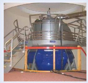
The magnet for a very high field - 22.3 Tesla - NMR instrument.
